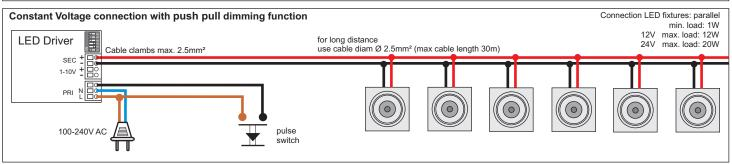
Always disconnect the mains of the LED driver before plugging or unplugging the LED's !! The LED's will be damaged or destroyed because of the high voltage present on the driver output when there is no load connected. Connect the main after all Led's and plugs are connected!
