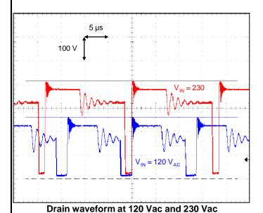
500 ns  $V_{IN} = 265 V_{AC}$   $V_{PK} = 462 V$   $V_{IN} = 230 V_{AC}$   $V_{PK} = 414 V$   $V_{IN} = 120 V_{AC}$   $V_{PK} = 256 V$
