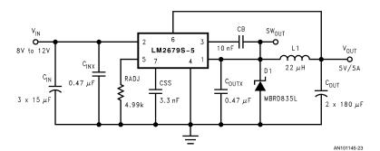
FIGURE 10. 5V/5A Design Circuit
