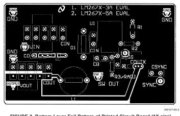
FIGURE 3. Bottom Layer Foil Pattern of Printed Circuit Board (1X size)
