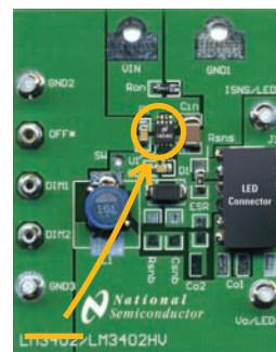
LM3402/02HV evaluation board with female 6-pin SIP connector and two standard 94 mil turret connectors for easy connection to LED array
