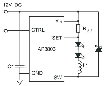
Figure 1: Typical Application Circuit
