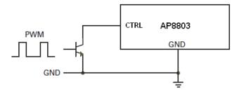
This scheme uses the 200k resistor between the CTRL pin and the internal voltage reference as a pull-up resistor for the external transistor eg MMBT3904.
