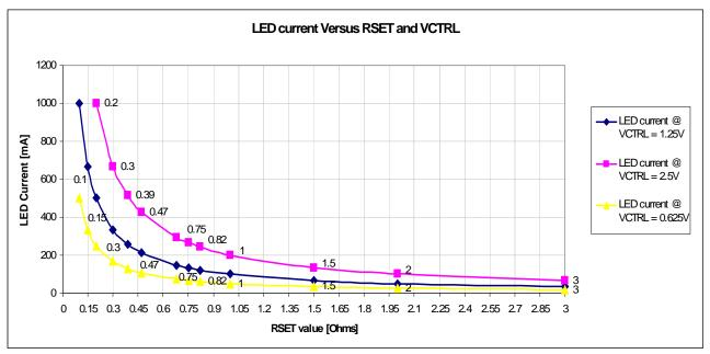
Figure 2: LED Current setting Vs RSET and VCTRL
