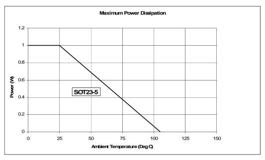
Figure 4: Derating curve
