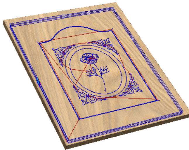
3D Preview showing the calculated toolpaths
