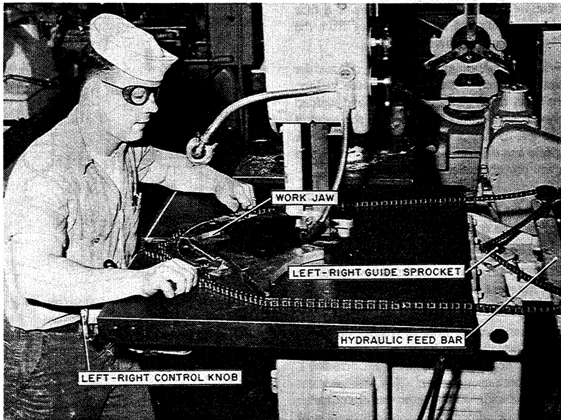
Figure 4-18.—Work jaw and feed chain adjustment.
