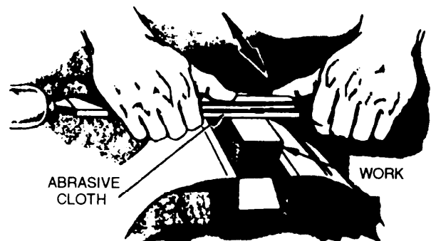
POLISHING METAL WITH ABRASIVE CLOTH WRAPPED AROUND A FILE
