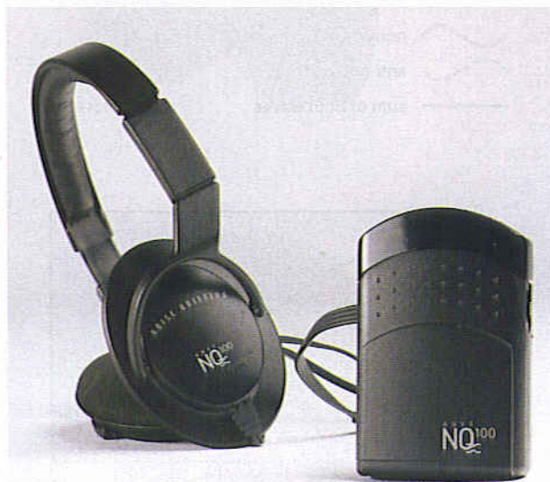
Figure 6. Typical low-cost ANR headphones for listening to music in noisy environments. The electronics box is connected to the signal source (personal stereo etc.) and linked to the headphones, which also include two microphones, using an 8-core screened cable.
