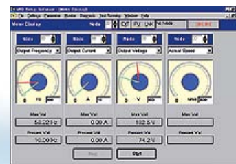
Display of system status values such as the PLC current frequency
