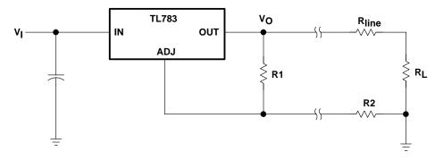
Figure 16. Regulator With Current-Set Resistor
