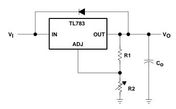
Figure 15. Regulator With Protective Diode
