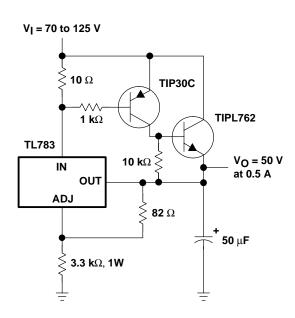
Figure 19. 50-V Regulator With Current Boost
