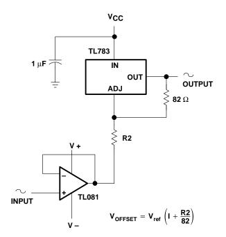
Figure 23. High-Voltage Unity-Gain Offset Amplifier
