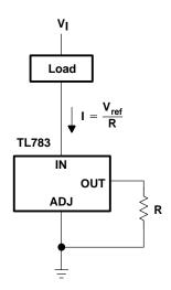
Figure 21. Current-Sinking Regulator
