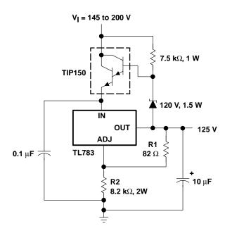
Figure 18. 125-V Short-Circuit-Protected Off-Line Regulator
