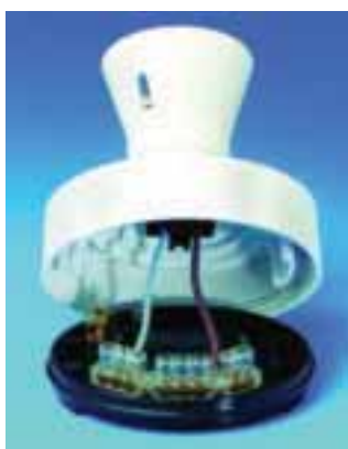
Pendant lamp holder has integral cord grip to prevent cable pull on terminals
