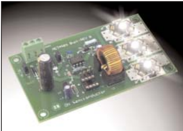
MC34063 Buck Demo Board from ON Semiconductor
