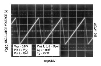
**Figure 3. Timing Capacitor Waveform**
