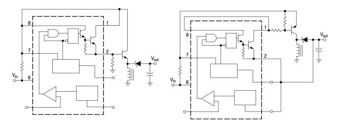
Figure 13. External Current Boost Connections for I<sub>C</sub> Peak Greater than 1.5 A
