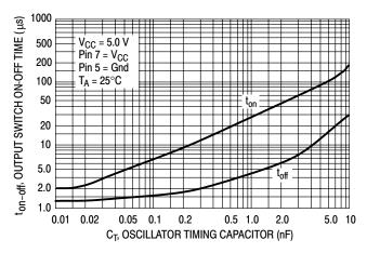
Figure 2. Output Switch On-Off Time versus Oscillator Timing Capacitor
