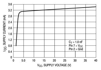
Figure 7. Standby Supply Current versus Supply Voltage
