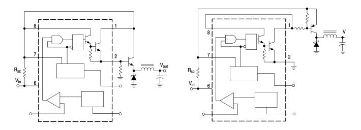
Figure 11. External Current Boost Connections for  $I_{\mbox{\scriptsize C}}$  Peak Greater than 1.5 A
