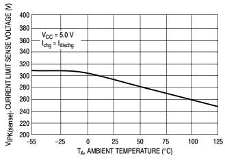
Figure 6. Current Limit Sense Voltage versus Temperature
