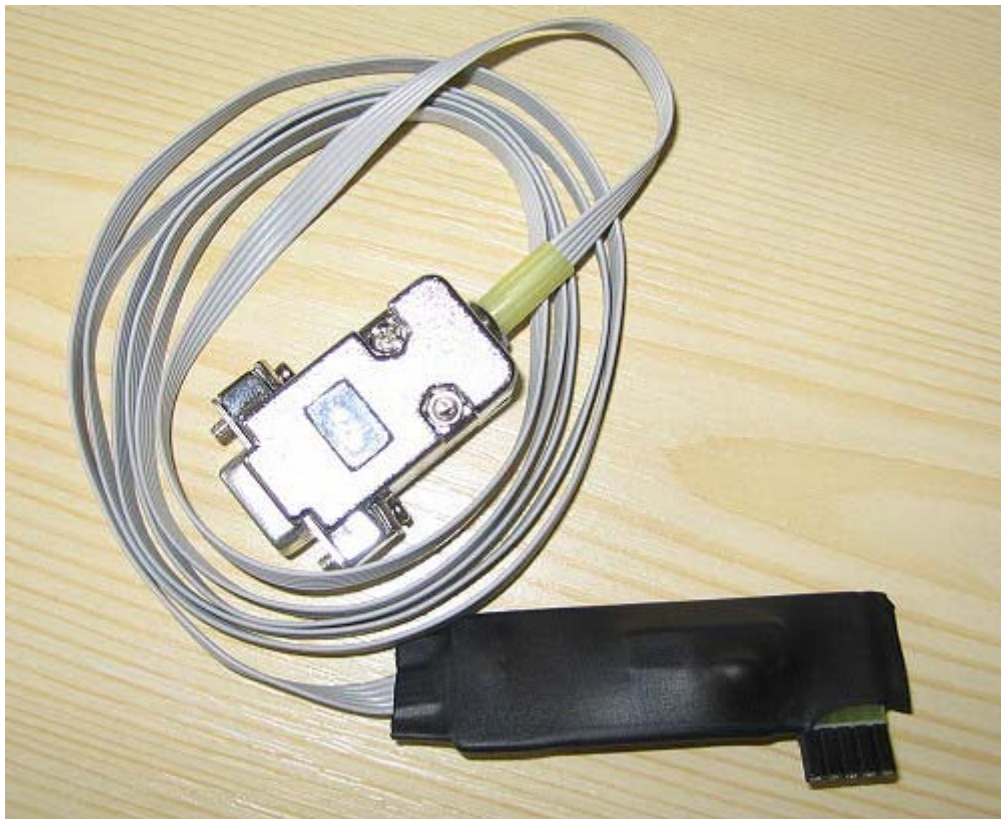
(Profi2S Servo Monitor adapter, RS232C)
