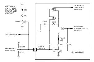
At anytime the operator can push the switch to the "STOP" position to immediately halt the G340 drive. Anytime the G340 is in the "FAULT" state (FAULT LED lit), all switching action stops and the motor freewheels and is unpowered. This will light the "FAULT" light.
