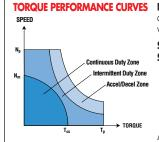
NOTE: Continuous torque specifications obtained with motor mounted to an 10"x10"x.25" aluminum plate at 25 C° ambient. Typical values are within ±10% of rating.
