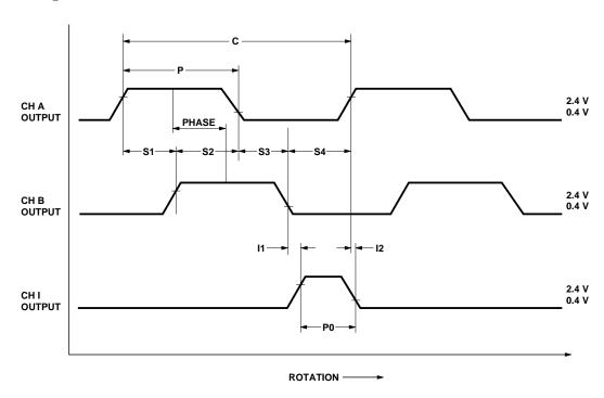
**Waveforms for Encoders without Line Drivers.**
