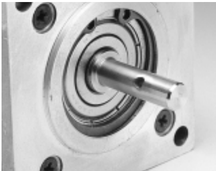
Cross-drilled shaft accepts hardened roll pin to attach sleeves, pulleys and gears.
