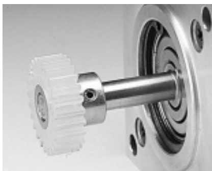
Plastic gear with brass bushing attached by hardened roll pin through cross-drilled hole in shaft.
