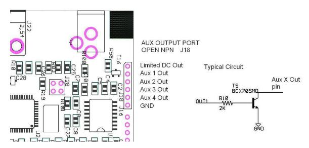
Figure 4-10. Auxiliary Output Port and drive circuit.
