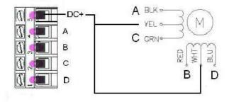
Never run the steppers without an inline fuse between the DC Motor Power supply and the MC433 – Power MOSFETs can fail and when they do they typically fail in a shorted state. Ensure there is a good ground between the DC Motor Controller, Board Logic Power and the controlling PC – the MC433 is a non-isolated design. All attached equipment must be at a common ground potential. Do not defeat the ground lug of all AC cords.
