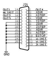
Figure 2-1. Parallel port signal function assignment.
