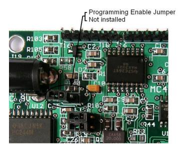
**MC433Prog.exe** is a command line program running under Windows98, 2000 and XP. The program emulates the operation of **ISProg.exe** (an AVR ISP programming utility) and is used to download new Flash and/or EEPROM files to the Motor Controllers and G Code Processor. **MC433Prog.exe** can be used to program each of the four processors individually or (using a command file) perform a sequence of programming functions on all four motor controllers in one pass.
