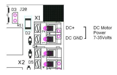
Figure 4-6. DC Motor Power Connector.
