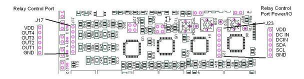
Figure 4-9. Relay Adapter connectors.
