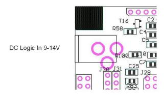
Figure 4-7. Board Logic Power Connector.
