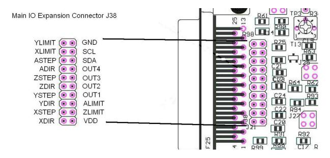
Figure 4-3. Main IO pin assignment.
