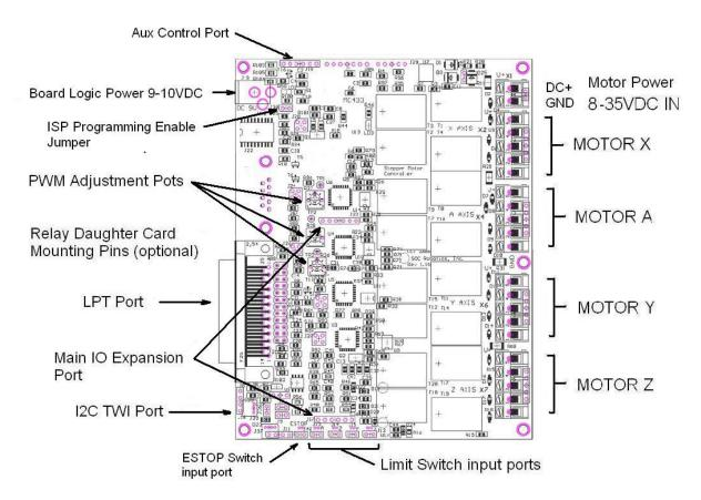
Figure 3.1. MC433 Top Side Connector Layout.
