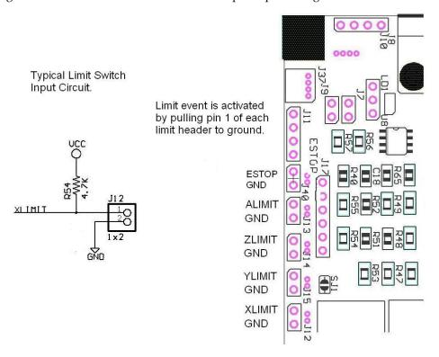
Figure 4-8. Limit Switch input ports.
