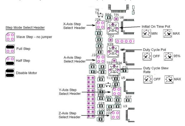
Figure 4.5. Step Sequence Selection and PWM Potentiometer settings.
