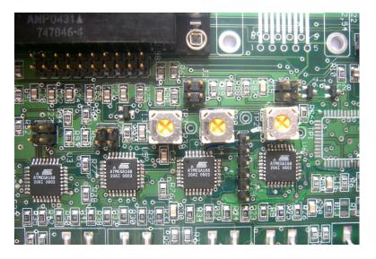
Figure 4.6. Step Sequence and PWM Potentiometers.
