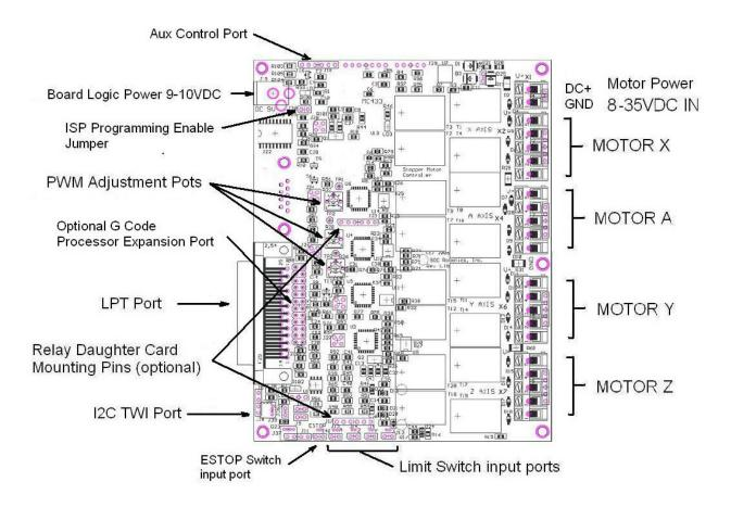
Figure 4-1. MC433 Expansion Connector locations.
