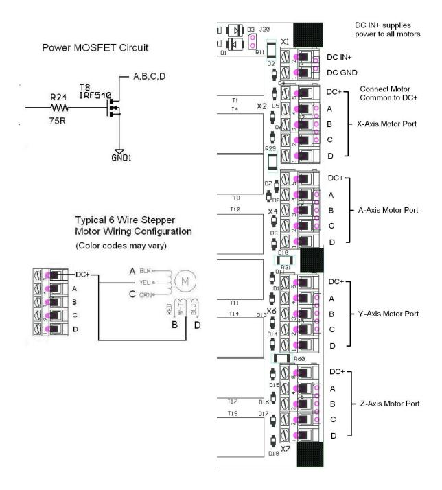
Figure 4-4. Stepper motor output drive ports and Motor Power In.
