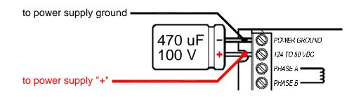
The power supply voltage must be between 24 VDC and 80 VDC. Beyond that, the choice of voltage is dependent on the application and the motor used. The power supply voltage should be between 3 to 25 times the motor's rated voltage. If it is less than 3 times, the drive may not operate smoothly and motor heating is excessive if it is more than 25 times the motor's voltage.
