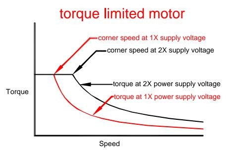
The result now is a two-part speed-torque curve which features constant torque from zero speed until it intersects the motor's natural load line, called the corner speed, beyond which the motor is in the constant power region.
