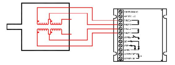
For a full-winding connection, the center tap is ignored and both end wires are used. The term "full-winding" is exactly equivalent to "series" connected while "half-winding" is virtually identical to "parallel" connected. The choice between the two is application dependent, which is discussed
