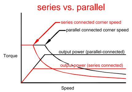
This shows a half winding connected motor delivers twice as much power as a full winding connection at a given power supply voltage. This is because full-winding inductance is four times higher than the half-winding inductance.
