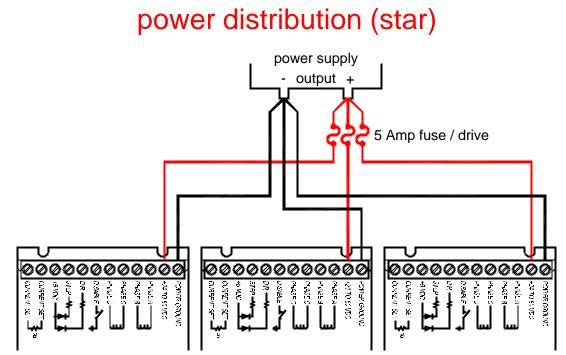
When using multiple drives from a common power supply, use individual supply and ground wires to each drive and return them to a common point back at the power supply. This is called a "star" power supply distribution; never ever use a "daisy-chain" power distribution, where the supply and ground wires for the next drive are picked up from the previous one.
