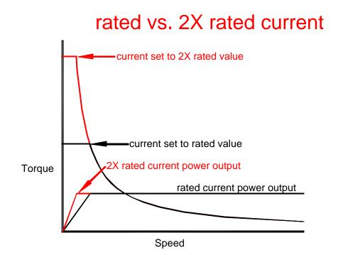
What can be seen is there is no increase of power output; the motor simply reaches its maximum power at a lower speed, all at the great expense of a four-fold increase in motor heating.
