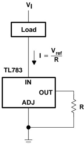
Figure 21. Current-Sinking Regulator
