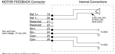
**Resolver Input Connections**
