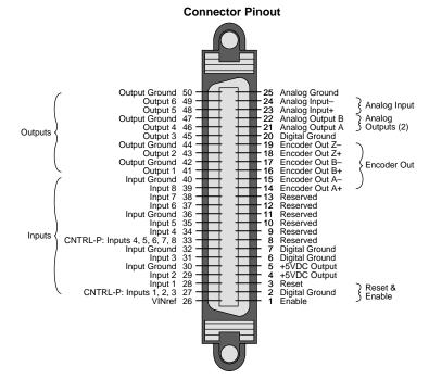
This section describes all inputs and outputs (I/O) located on the 50 pin DRIVE I/O connector. The connector pinout is shown in the next drawing.
