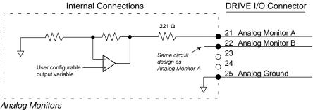
You can configure the analog outputs to monitor many different variables, such as current, velocity, temperature, etc. You can also scale the outputs. See the DMON commands in *Chapter 3 Configuration* and the *Gemini Programmer's Reference* for more information.
