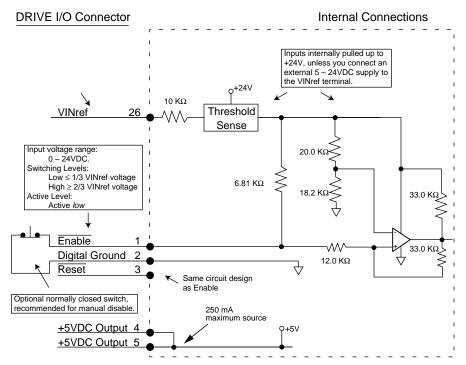
Enable Input and Reset Input
