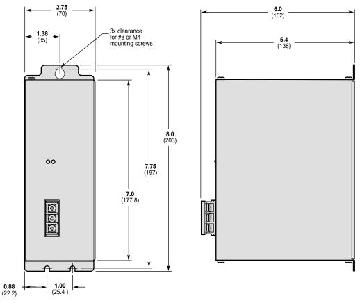
Dimensions – GPDM Power Dissipation Module
