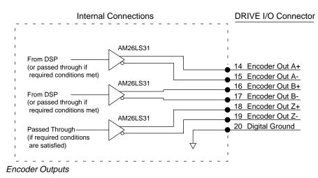
You can use the ORES command to configure the encoder outputs.
