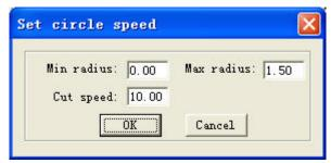
When the radius of circle is in the range between "Min radius" and "Max radius", the cut speed will automatically be changed to the number of "Cut speed".
