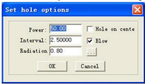
**Power:** the laser power when a layer is processed.
