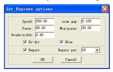
**Speed:** engraving speed on X-axis.
