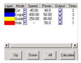
In the "Output" column, you can select that the current layer is output or not.
