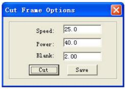
**Speed:** you can choose different speed according to different material. It's better to confirm proper speed through testing.
