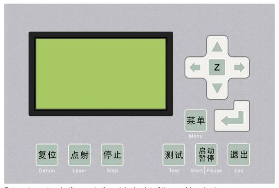
Datum: Laser head will move to the original point of the machine slowly.
