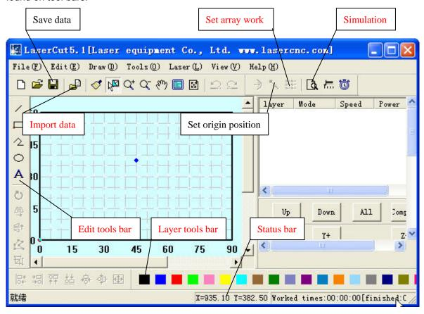
Let mouse stay on an icon for a moment, and it will show the explanation of basic function of tools bar. The following is the explanation of all tool bars.
