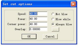
Speed: vector speed on X-Y axis
