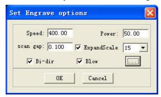
**Speed:** engraving speed on X-axis.
