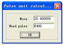
**Move:** When the stepping motor moves a circuit, the laser head will move a relative length. You need to input the number in it.
