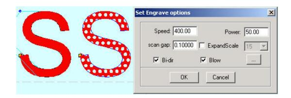
The right "S" is the result of selecting "Fill circle". You can change the radius and space by inputting different parameters.
