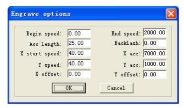
**Begin Speed and End Speed:** When the engrave speed is set in the range between Begin Speed and End Speed, the system will automatically apply the numbers of Acc Length, Backlash...
