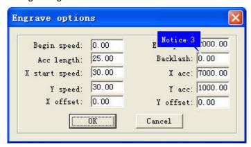
The best way is single direction engraving. But this will slow down the efficiency. Parameters should be set as the following dialog box.
