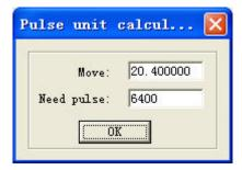
**Move:** When the stepping motor moves a circuit, the laser head will move a relative length. You need to input the number in it.
