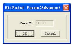
Power2: laser power of the second laser head. This needs hardware support.
