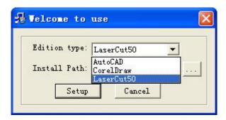
There are three options in "Edition type". The default path is "C:\LaserCut50". Click and you can change the install path. Click "Setup" and the software will be installed.
