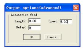
**Length (feeding length):** When input a certain number in it, feeding motor will give a certain space after every processing finished. This function needs hardware support.
