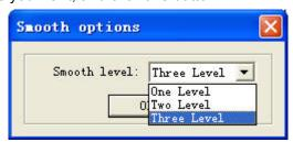
There are 3 options. Compared with "One Level" and "Two Level", "Three Level" is smoother. But the distortion is bigger than the others.
