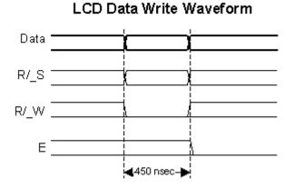
The interface is either a 4-bit or 8-bit parallel bus that allows fast reading/writing of data to and from the LCD.
