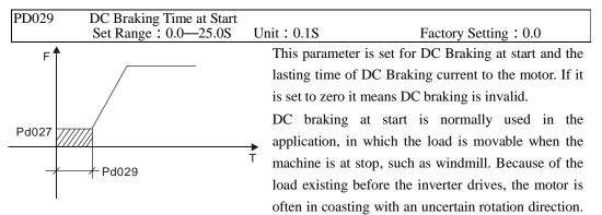
So the DC braking can be executed before starting the motor to prevent the inverter from tripping. This setting is valid only when PD025 is set to 0. For the related parameters refer to PD025, PD031 and PD027.
