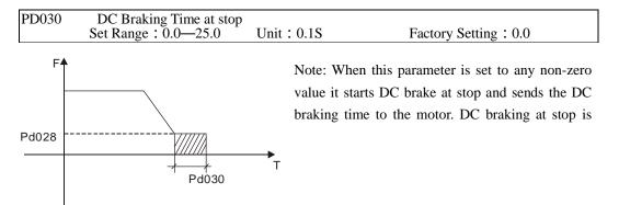
often used for a high-level stop or positioning control. When this parameter is set to zero it closes DC braking at stop.
