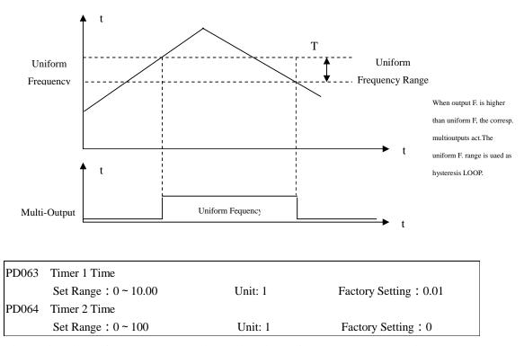
Timer 1 is a timer of  $0.1s \sim 10.0s$  and Timer 2 is a timer of  $1s \sim 100s$ . When the timer start at multi-inputs is closed (on) the timer starts to count time. When it reaches the set time the corresponding multi-output contact will act. When the timer start is opened (off) the timer time at the multi-output will be reset.
