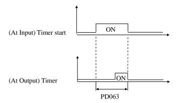
For example, set PD063=5.0s. When the external control terminal (Multi-Input) is valid the output terminal will be valid after five (5.0) seconds, the signal of which can be used to control other corresponding signals.
