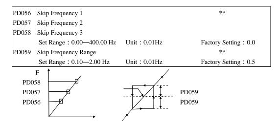
These three frequency skipping points are set for avoiding a mechanical resonance point. In case of PD059=0, all skip frequencies are invalid. The actual skip frequency range is two times that of PD059, as shown in the above diagram.
