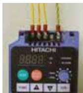
Input wiring for 3-phase input (models -NFU, -LFU, -HFEF, -HFU)
