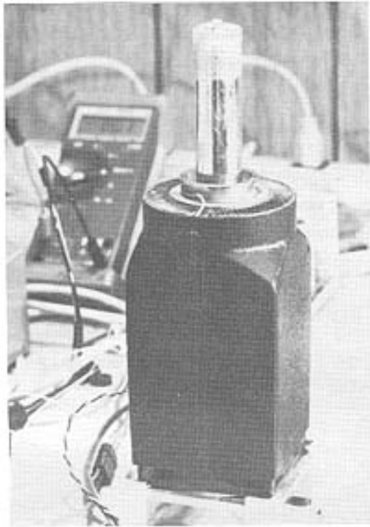
Figure 7 - Small cryocooler capable of lifting 4.0W at 77K (developed for high temperature superconductor applications)
