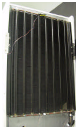
Figure 3 - External condenser for heat rejection
