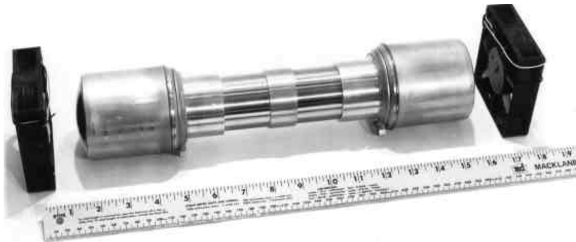
Figure 6 Horizontally Opposed Arrangement (Boxer)
