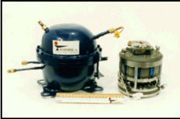
Figure 2 - Prototype linear compressor (on right) compared to same capacity conventional compressor
