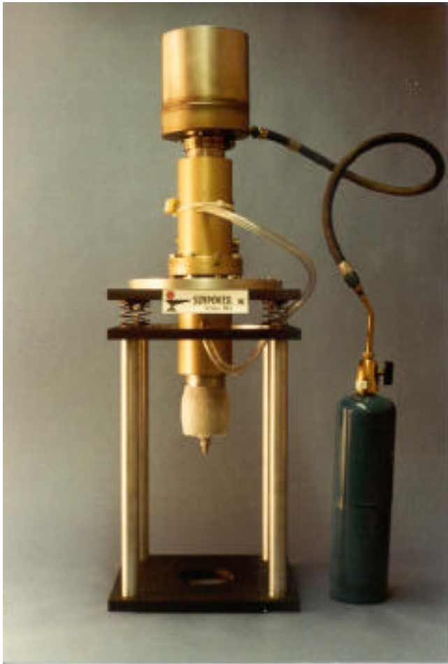
Figure 2 – Duplex demonstrator machine with recuperative combustor, note ice formation on cold end.
