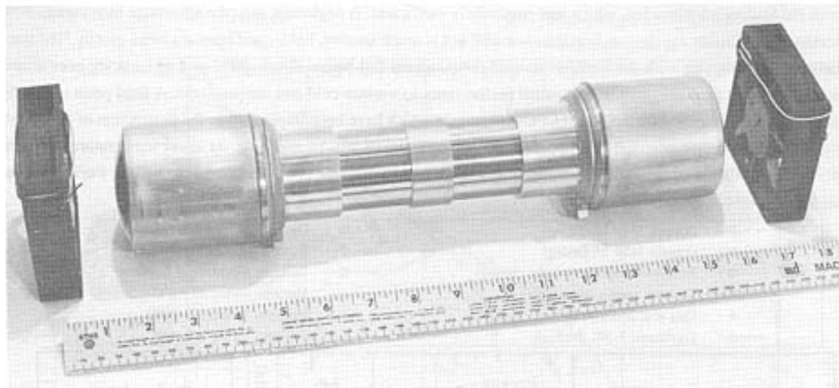
Figure 4 - General configuration of opposed free-piston Stirling cooler (cooling fans are at each end)
