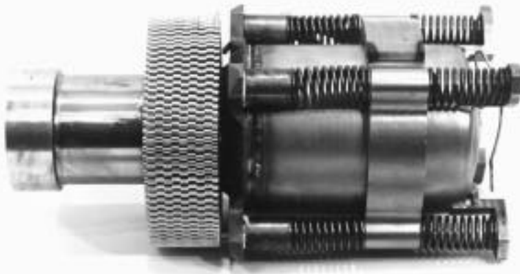
Figure 4 - Small free-piston Stirling cooler capable of cooling a 110 liter refrigerator
