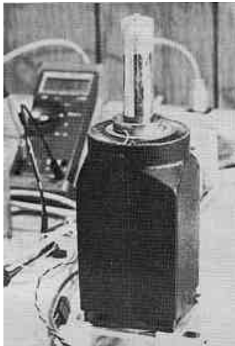
Figure 9 M77 Free-Piston Cryocooler. Lift 4 W at 77 K ( www.sunpower.com ).
