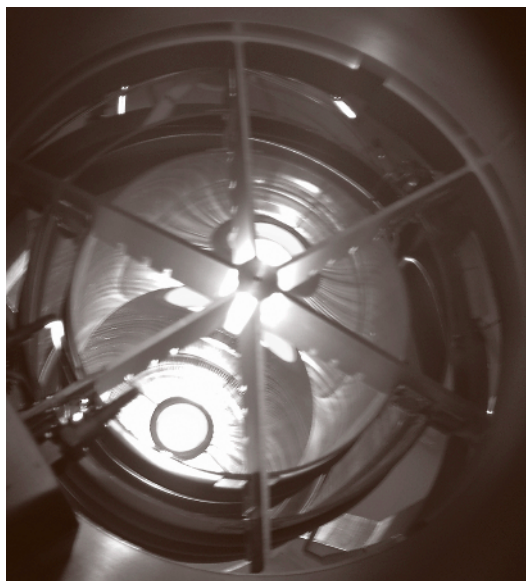
Fig. 11.176 EUV plasma source integrated into an optical system
