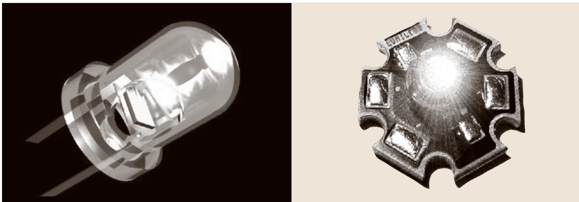
Fig. 10.16 Schematic of a classical indicator and high-power illumination LED
