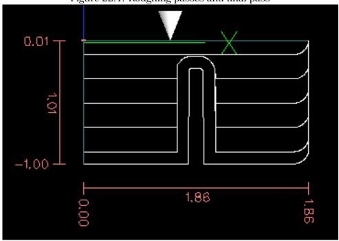
Figure 22.1: Roughing passes and final pass
