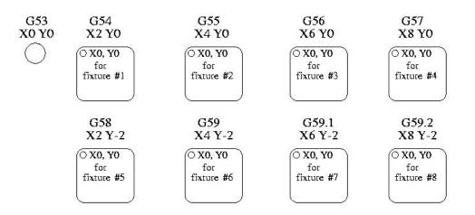
Figure 13.1: Fixture Offsets
