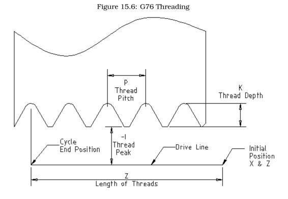
**Drive Line** A line through the initial X position parallel to the Z.
