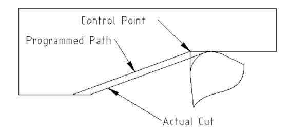
In the above example it is a simple exercise to adjust the programmed path to give the desired actual path by moving the programmed path for the ramp to the left the radius of the tool tip.
