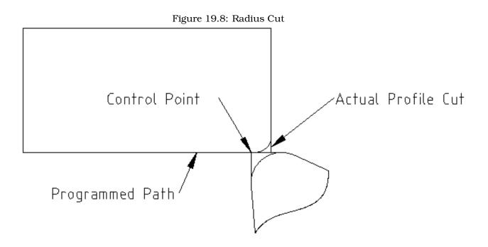
Now you can see as the control point follows the radius programmed the tool tip has left the part and is now cutting air.
