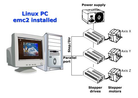
Figure 2.1: Simple EMC2 Controlled Machine
