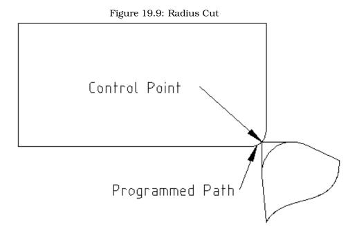
In the final figure we can see the tool tip will finish cutting the face but leave a square corner instead of a nice radius. Notice also that if you program the cut to end at the center of the part a small amount of material will be left from the radius of the tool. To finish a face cut to the center of a part you have to program the tool to go past center at least the nose radius of the tool.
