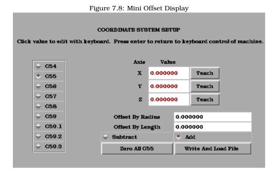
You can also teach using an edgefinder by adding the radius and length to the offset\_by widgets. When you do this you may need to add or subtract the radius depending upon which surface
