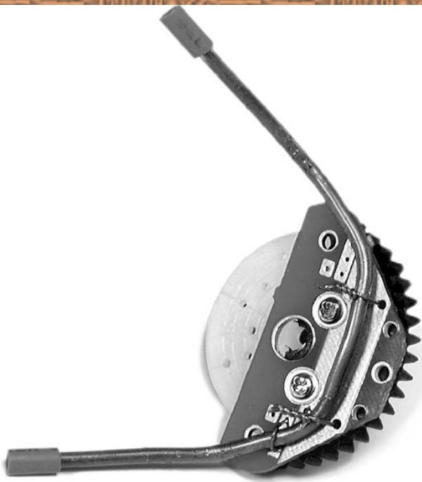
FIGURE 27: The completed back gear/leg assembly.
