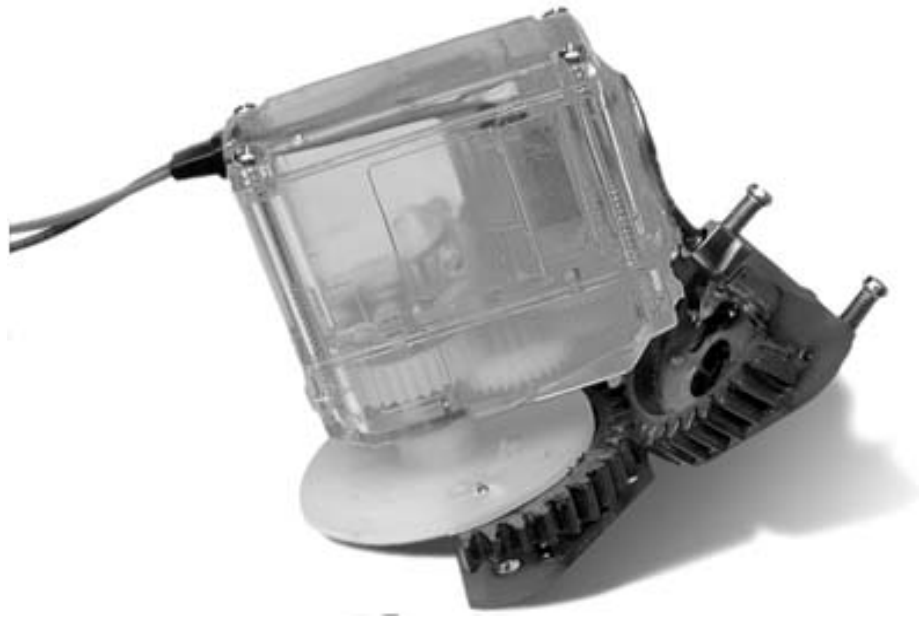
FIGURE 21: Test fitting to make sure that the drive gear and the idler gear mesh properly. Bend idler shaft down, if necessary.
