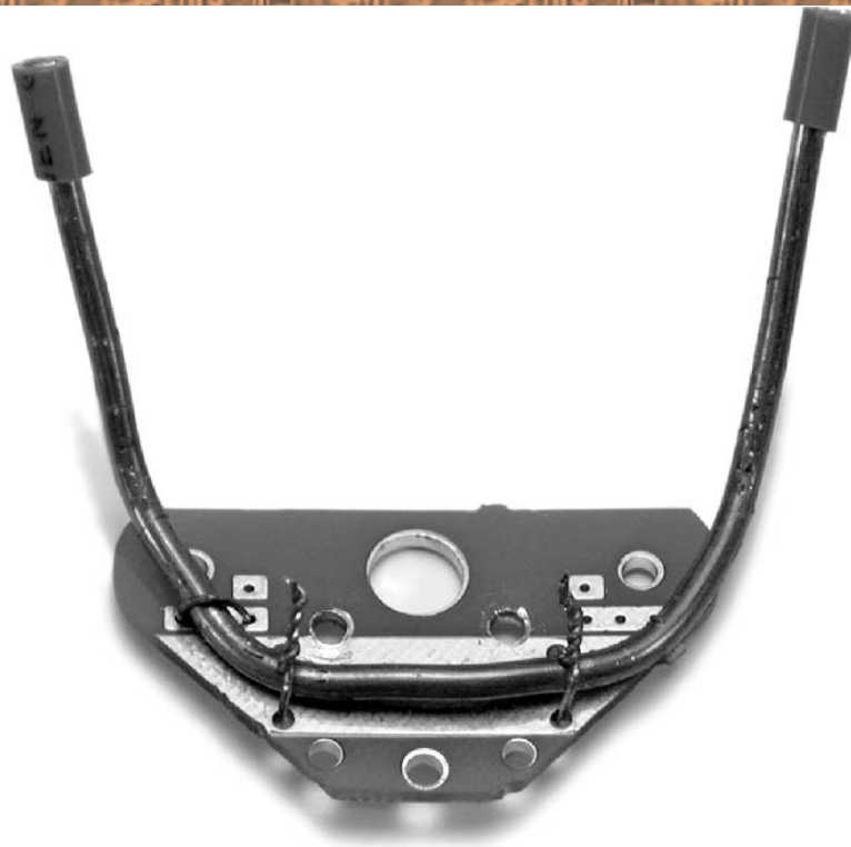
FIGURE 25: Back legs secured to LMP. Note third wire wrap (far left) to further secure leg.
