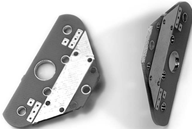
FIGURE 24: Solarbotics LMPs with their tips trimmed to fit our walker.
