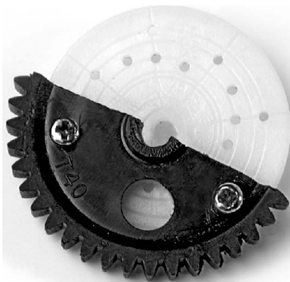
FIGURE 20: The drive gear mounted (here via screws) to the servo horn.
