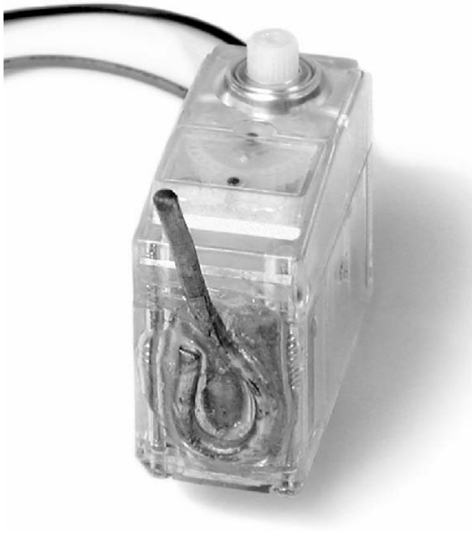
FIGURE 16: Our idler shaft glued to the motor casing (opposite of the drive shaft and motor wires).
