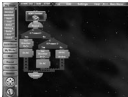
Figure 1.8 A Sample Stair-Climber Program Built with RIS 2.0
