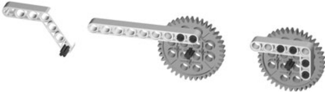
Figure 6.7 Avoiding Axle Torsion
