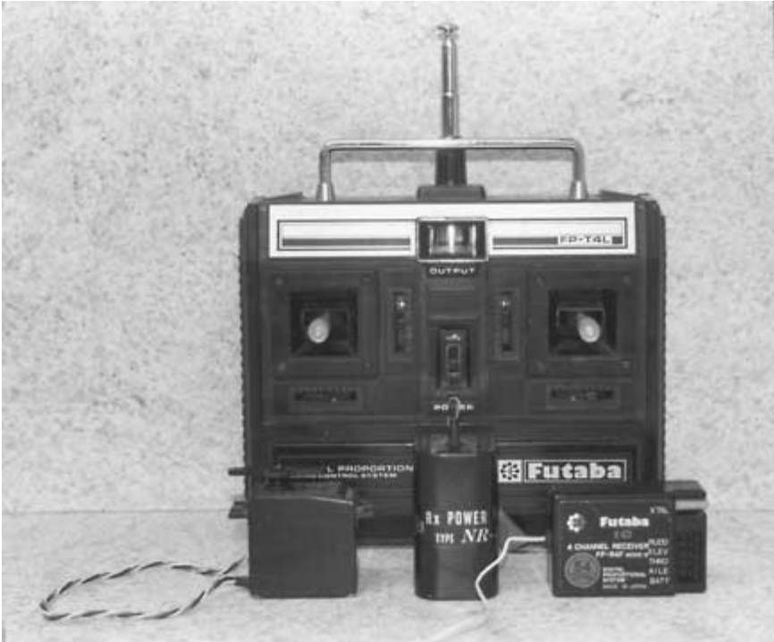
FIGURE I-15. Basic wireless remote control system.
