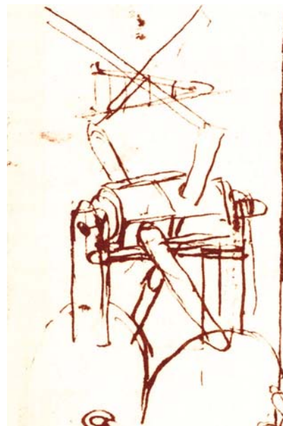
▲ Fig. 2.17. CA, f. 296 v-a [812 r]. Escapement mechanism detail
