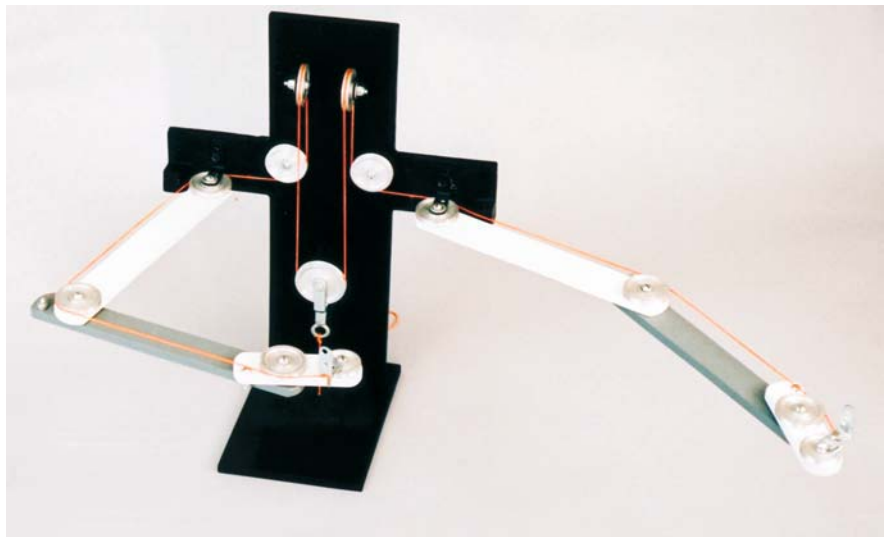
Fig. 3.56. Robot Knight cable system differential motion of arms
