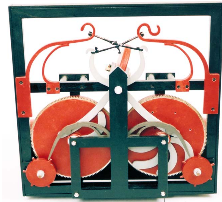
Fig. 2.51. Left turn produced by no cam
