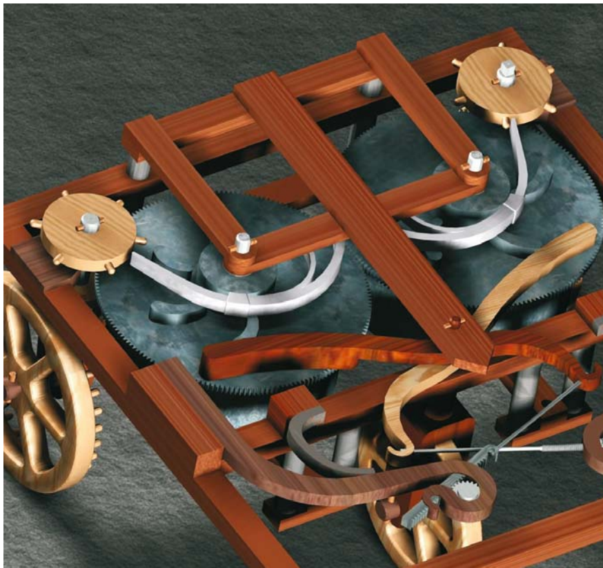
Fig. 2.44. Array of cams attached to the top of the large barrel gears controls the direction and velocity of the automaton
