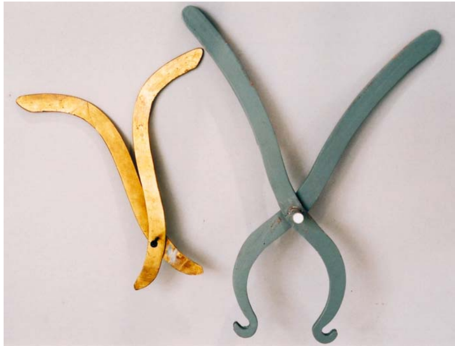
Fig. 4.51. Bottino trigger linkage ( left ) programmable automata linkage ( right )
