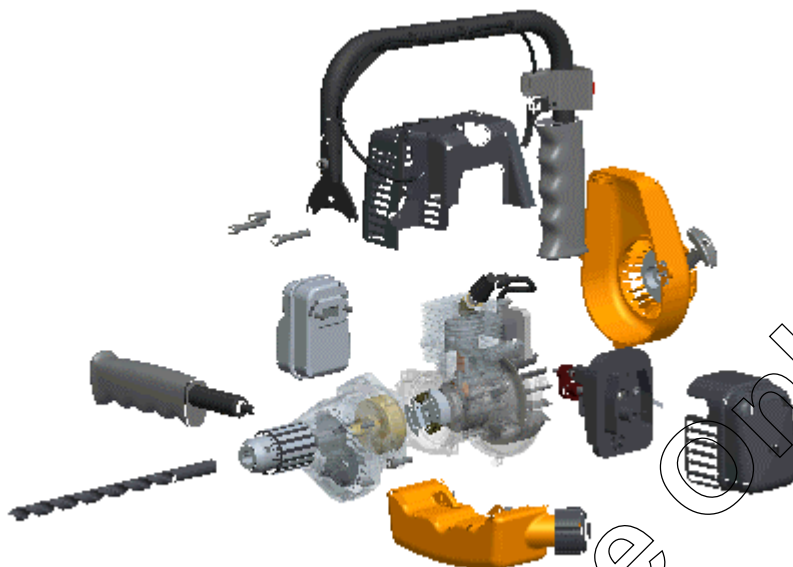
Figure 45: Creating the Main Handle/Gearbox Bolts Explode State
