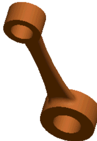
Figure 5: Replacing Sketched Entities (left) and the Completed CONNECTING_ROD.PRT (right)
