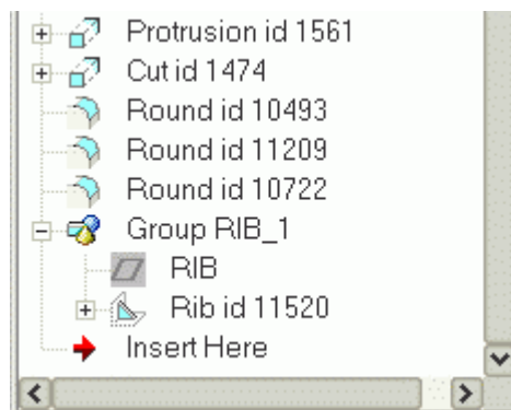
Figure 25: Model Tree and Completed Rib Feature on RECOIL_COVER.PRT
