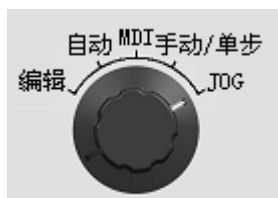
mode selection: edit, auto, MDI, handwheel or single step, JOG
