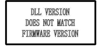
**Reason**: the DLL used to generate the processing file dose not match the firmware. **Solution**: see 10.1
