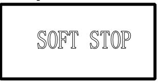
**Reason**: figure to process is beyond the range of the worktable. Usually it happens when the laser head datum and there is no correct docking point for the laser head in the case of immediate output.
