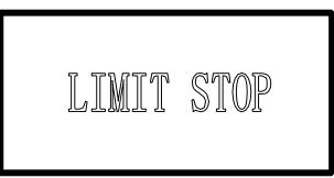
**Reason**: user checks the immediate output when the laser head doesn't datum, and then the processing range is beyond the worktable and stop when it gets limit signal. It will also happen when there are interruption signal due to the sophisticated surrounding.
