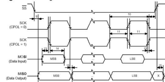
In principle the timings are the same in slave mode like previously described in master mode. Because of the switching of the roles between master and slave the requirements on the timing are inverted as well. The minimum times of the master mode are now maximum times and vice versa.
