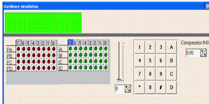
The top section is a virtual LCD display. It works for display code in PIN mode and bus mode. For bus mode only 8-bit bus mode is supported by the simulator.
