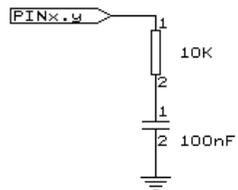
The capacitor is charged and the time it takes to discharge it is measured and stored in the variable. So when you vary either the resistor or the capacitor, different values will be returned. This function is intended to return a relative position of a resistor wiper, not to return the value of the resistor. But with some calculations it can be retrieved.
