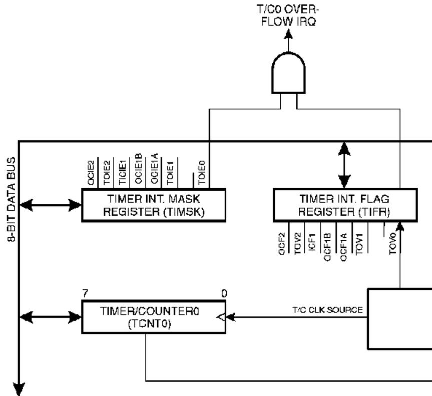
The 8-bit Timer/Counter0 features both a high resolution and a high accuracy usage with the lower pre-scaling opportunities. Similarly, the high pre-scaling opportunities make the Timer/Counter0 useful for lower speed functions or exact timing functions with infrequent actions.
