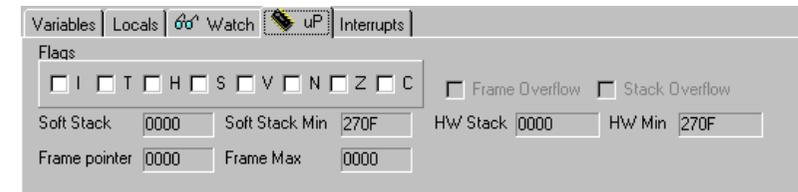
This TAB shows the status of the microprocessor SREG register.
