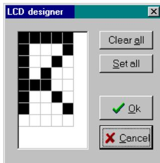
The LCD-matrix has 7x5 points. The bottom row is reserved for the cursor but can be used. You can select a point by clicking the left mouse button. If a cell was selected it will be deselected.
