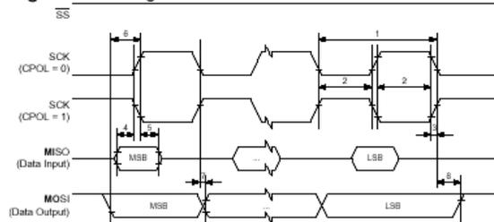
The minimum timing of the clock signal is given by the times "1" and "2". The value "1" specifies the SCK period while the value "2" specifies the high / low times of the
