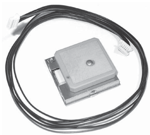
Figure 13-3: A long GPS-receiver-to-shield cable
