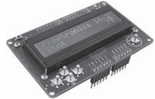
Figure 13-6: The Freetronics LCD & Keypad shield
