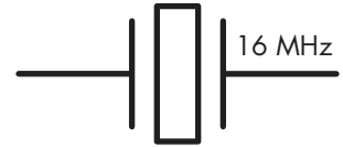
Figure 11-4: Crystal oscillator schematic symbol
