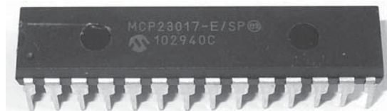
Figure 17-5: Microchip Technology's MCP23017 port expander IC
