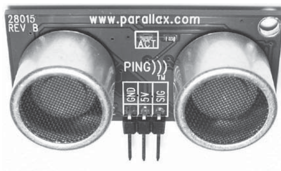
Figure 12-26: The Ping))) ultrasonic distance sensor
