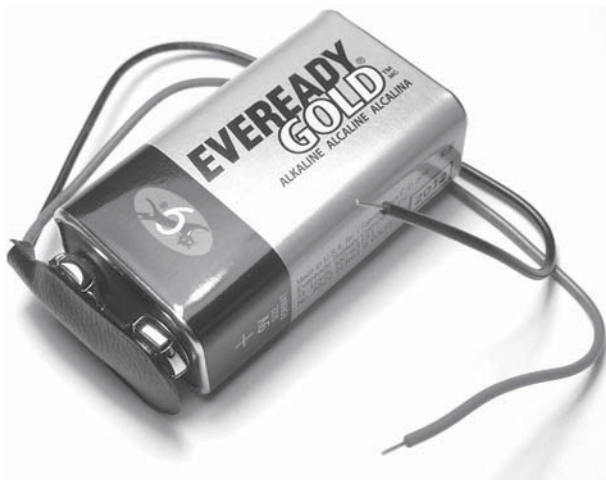
Figure 11-9: 9 V battery and snap connector
