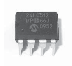
Figure 17-2: Microchip Technology's 24LC512 EEPROM
