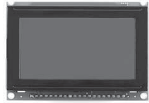
Figure 7-8: A graphic LCD module
