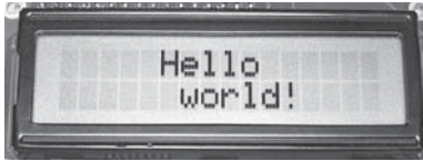
Figure 7-3: LCD demonstration: "Hello world!"
