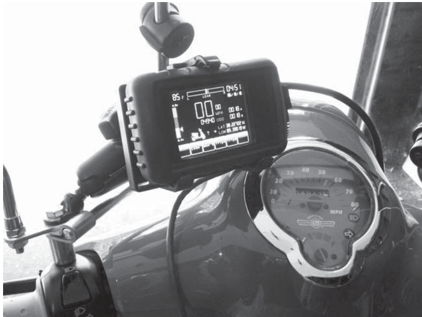
Figure 1-4: The Scooterputer display (courtesy of Kurt Schulz)
