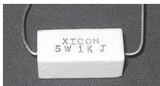
Figure 3-5: A 5-watt resistor
