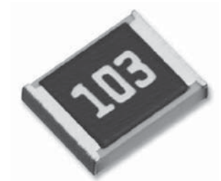
Figure 3-3: Example of a surface-mount resistor
