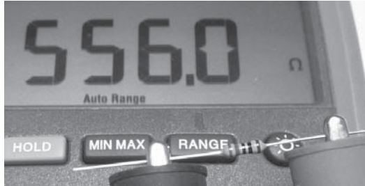
Figure 3-4: Multimeter measuring a 560-ohm 1 percent tolerance resistor
