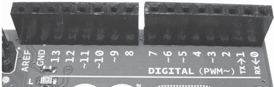
Figure 2-5: The digital input/output pins
