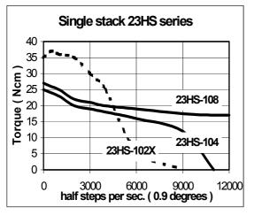
Bi-polar drive with coils in parallel
