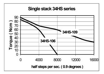
Bi-polar drive with coils in parallel
