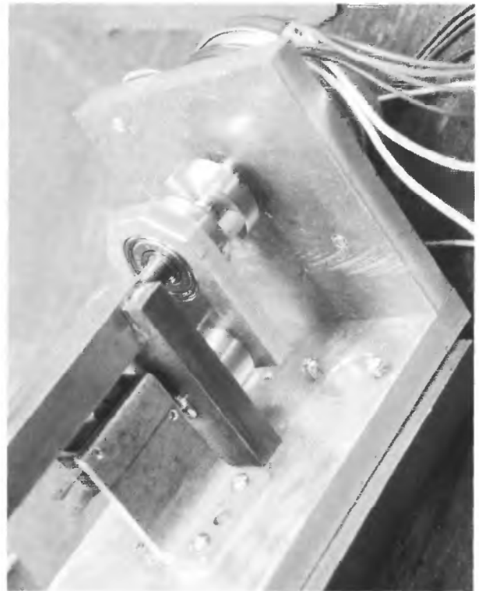
Reg Miller used a brass guide tube and brass brackets, but all the other parts were aluminum. Note the precision roller bearing and also the coupling rods made from rubber.
