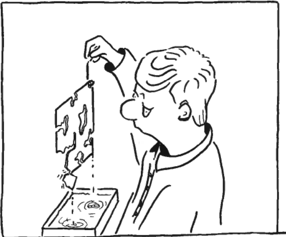
Figure 3.1 The chemicals used in making circuit boards require proper temperatures to work effectively...
