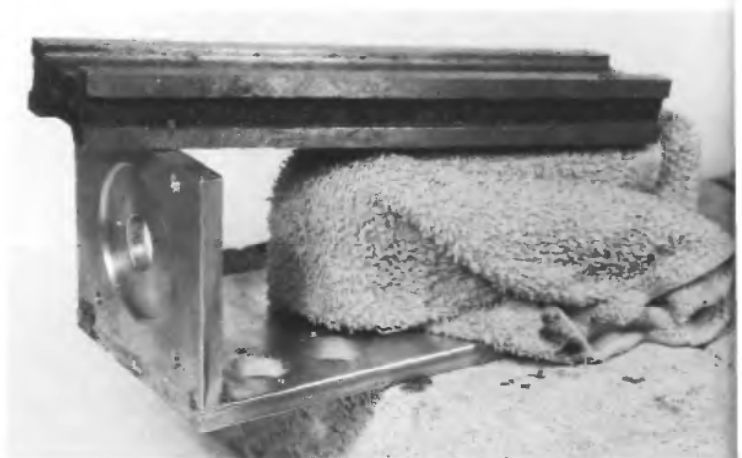
Setup for soldering the top and back plates together. The space bar held everything square and the damp cloth prevented the previous soldering job from melting.
