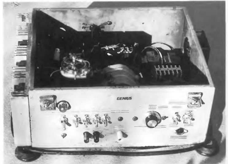
1.4. A recycled relay box from a stone crushing control panel served Remie Grimminck well for his EDM.
