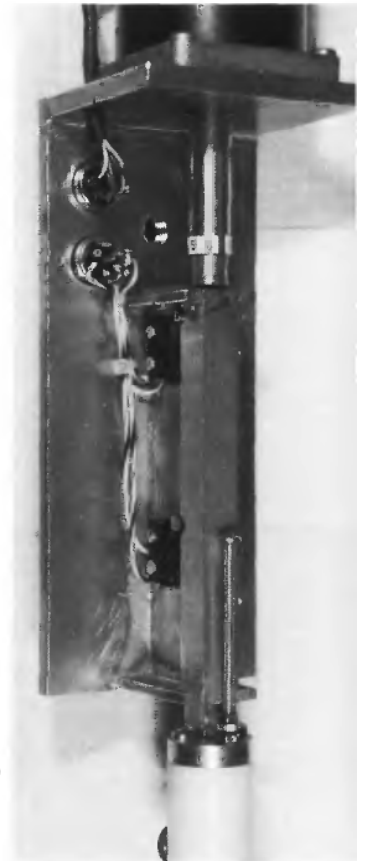
The author's second go at the head, this time using a 200-step motor and a 40 TPI leadscrew. If the lower guide bracket were the same size as the top plate, then a simple sheet metal shroud could be securely fitted around the guide tube assembly.
