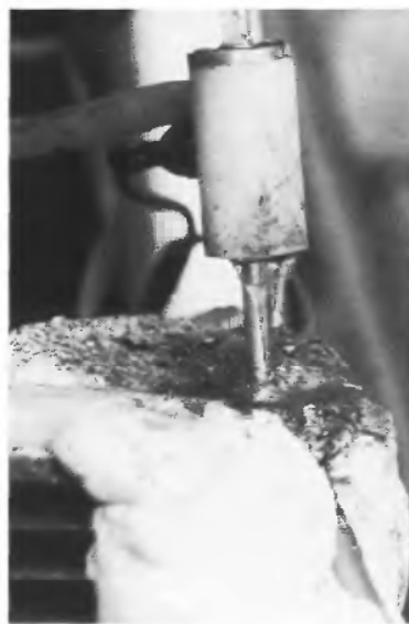
As the electrode eroded deeper into the hole, more effective flushing was needed. The tap water was then fed through a rubber hose into the hollow electrode.
