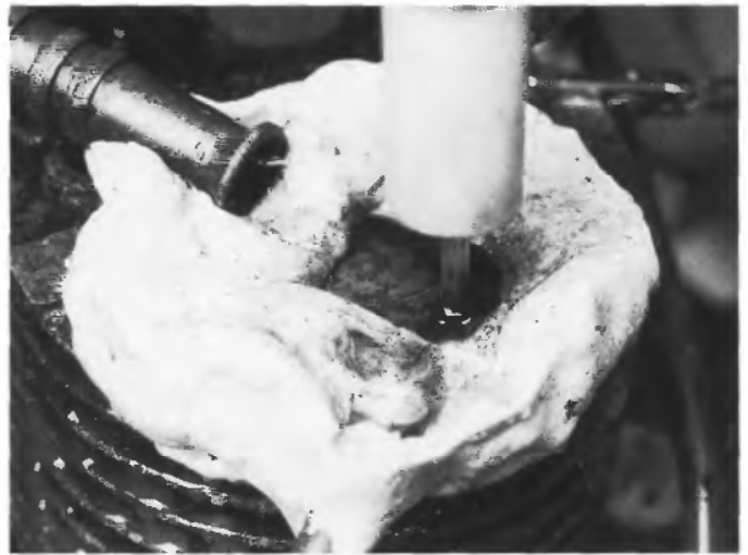
The garden hose supplied the dielectric (tap water) and putty kept the fluid contained and directed to the rubber drain.
