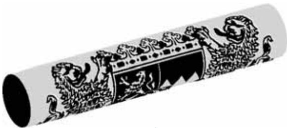
Complex engraving with picking out of the corners on an isel machine with 4th axis (rotary axis)
