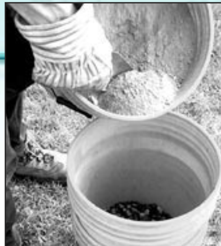
Add the ashes to the filter bucket
