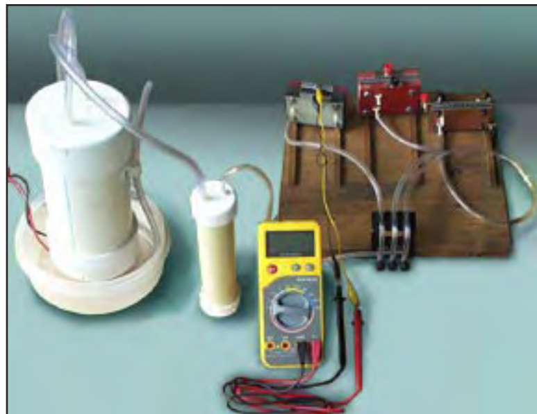
From left – electrolyzer, bubbler, meter and testing stand with 3 fuel cells.
