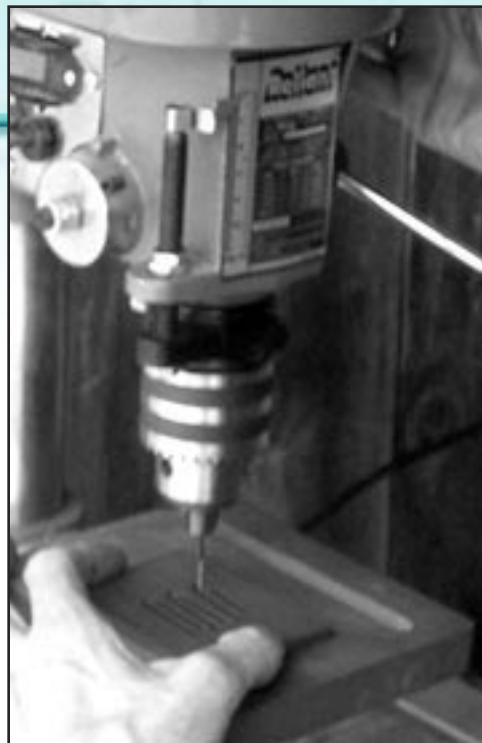
Routing the serpentine flow fields
