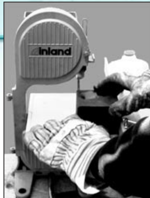
Cutting graphite blocks with wet band saw
