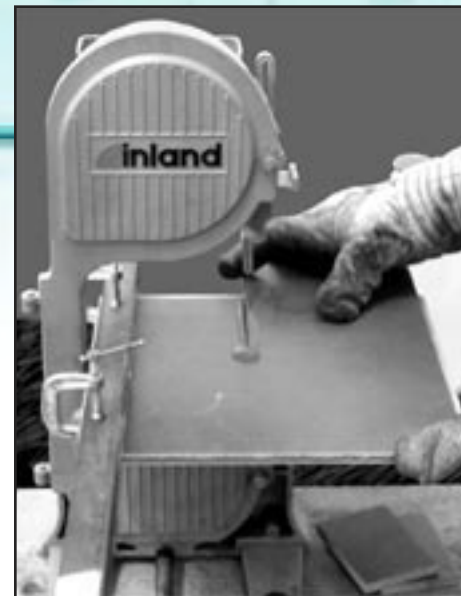
Cutting out fiberglass end plates
