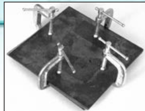
The MEA is clamped between the plates.
