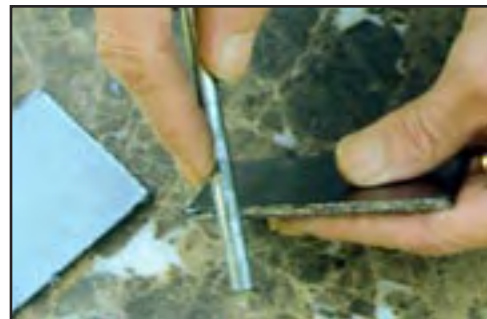
Smoothing the edges of the graphite plates with a smooth metal tool handle.
