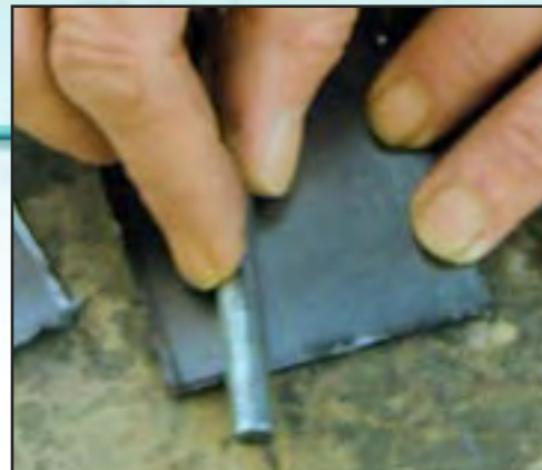
Smoothing the edges of the graphite plates with a smooth metal tool handle.
