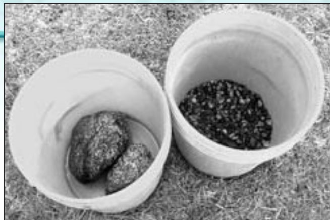
Drip bucket (left) and filter bucket
