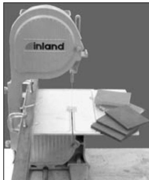
Wet and dry band saw
