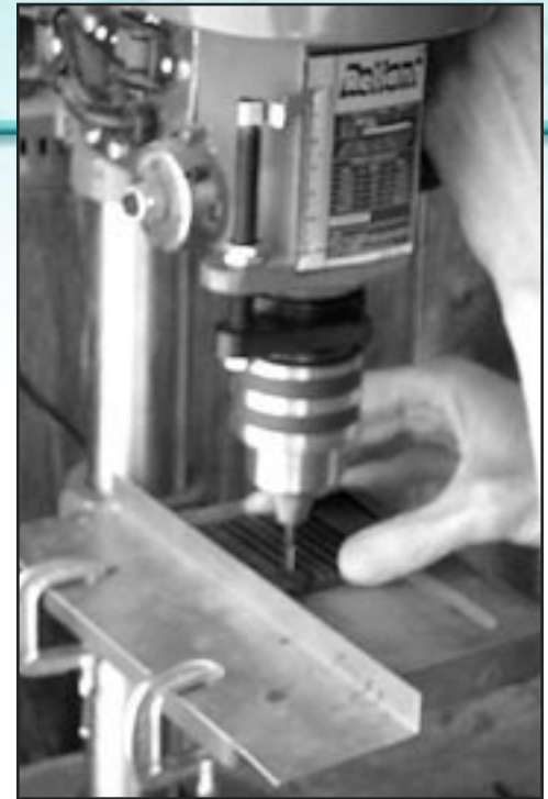
Routing the vertical flow fields
