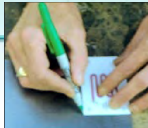
Using a template to mark the graphite foil.
