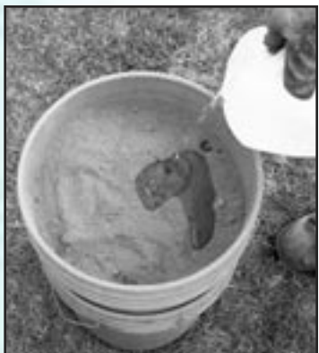
Add the water to the ashes. Filter bucket is set into drip bucket.
