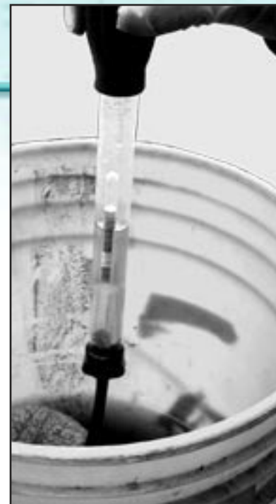
Testing the lye in the drip bucket with a hydrometer.
