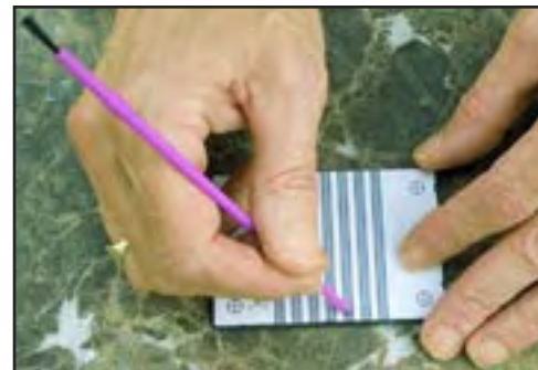
Marking the flow fields on the graphite plates
