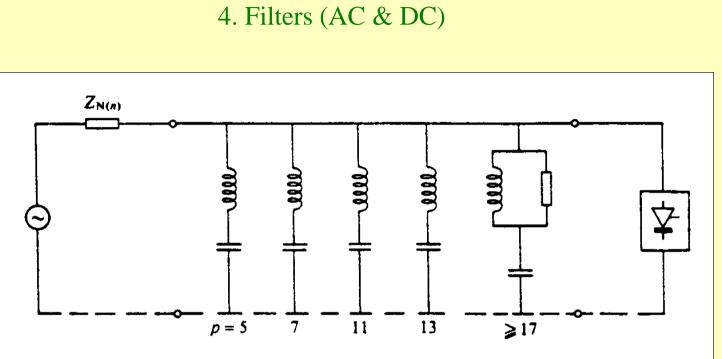
Principle : Each individual filter is turned to each harmonic (L, C) lots of no-load losses
