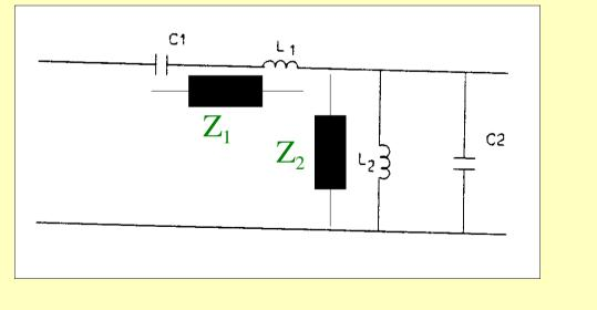
Series resonance filter (current filter)
