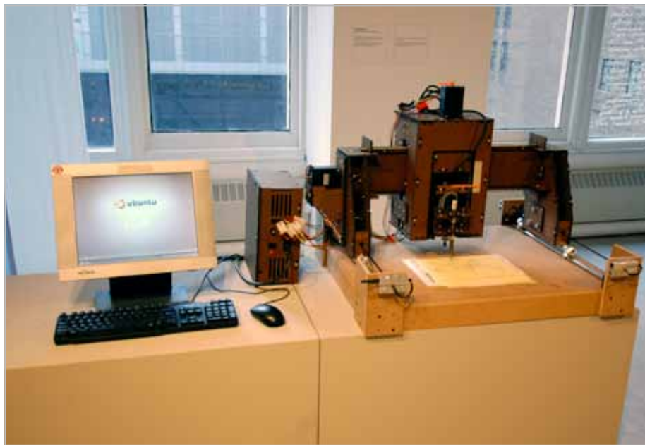
DIYLILCNC Components (Left to Right): Controller PC, Driver Board, Gantry/Mill.
