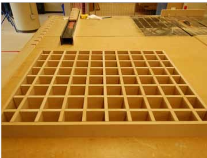
We added extra internal spans to our cutting bed.
