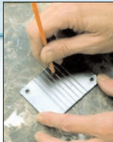
Making the flow fields with a paint brush handle
