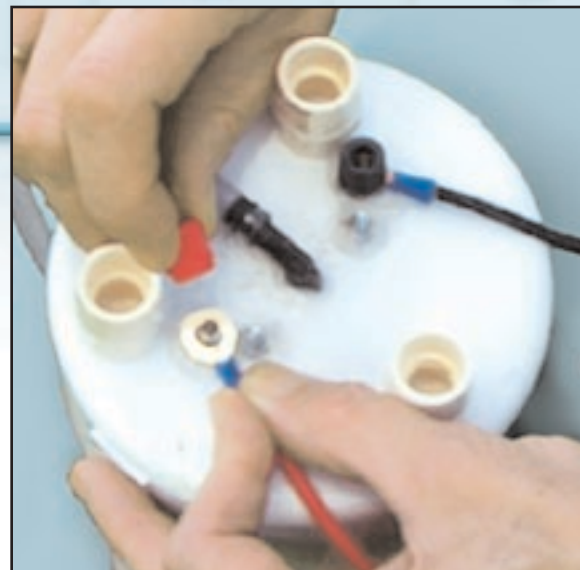
Attaching connections. The electrolyzer is upside down.
