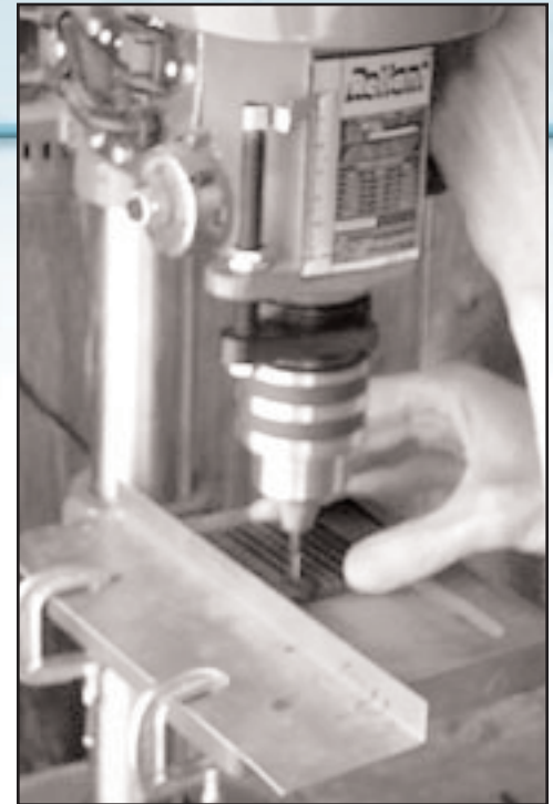
Routing the vertical flow fields
