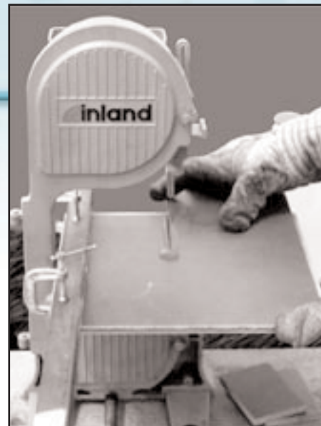
Cutting out fiberglass endplates
