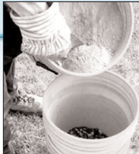
Add the ashes to the filter bucket
