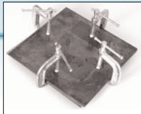
The MEA is clamped between the plates.
