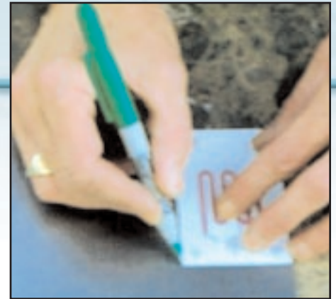
Using a template to mark the graphite foil.
