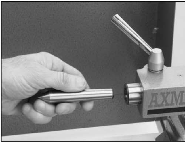
Inserting dead centre into tailstock barrel
